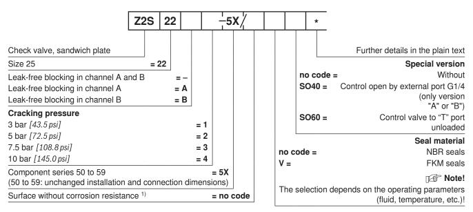
1) Corrosion-resistant surface upon request: e.g. "J50" thick layer passivated (DIN 50979 Fe//Zn8//Cn//T0)
